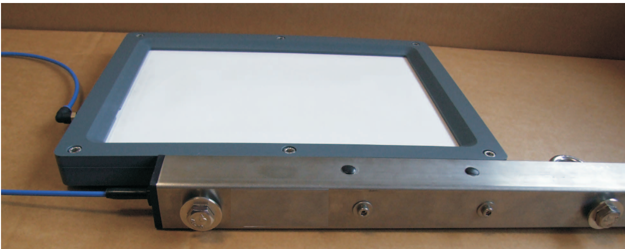
Figure 2 Installation of the filter membrane module on the slide
